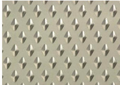
Also suitable for retrofitting: Honking silos can even subsequently be equipped with goffered plate.
